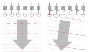
Figure 1:electronic beam-deflection, left: Boresight, right: Deflected
